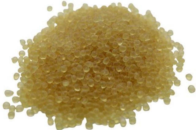
**FL80** - the pressure-sensitive hot melt adhesive is used for pressure-sensitive tapes and stock labels.
